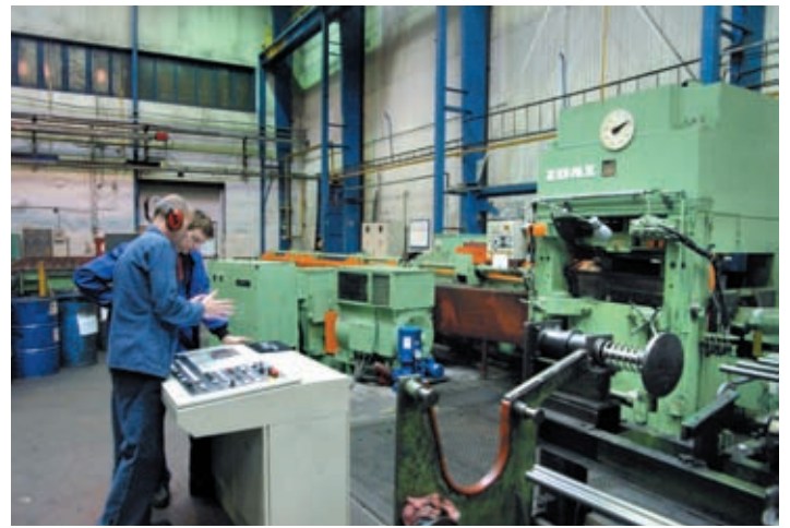
The XRK 2-80 polishing and straightening machine is designed for straightening and surface finishing of bars.
